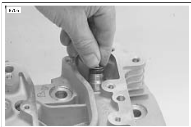
Figure 3-81. Valve Seal and Lower Collar Assembly Installation
