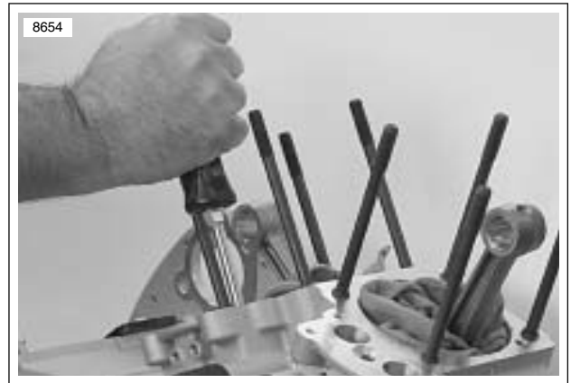
Figure 3-132. Checking Cam Gear End Play
