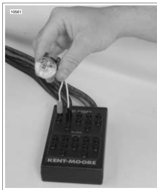
Figure 4-48. Testing Ignition Coil Connectors
