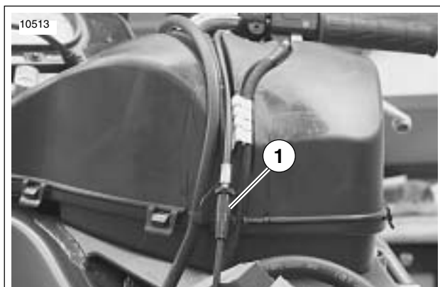
Figure 1-45. Checking For 1/8 in. (3.2 mm) Maximum Free Play In Either Direction For Proper Adjustment
