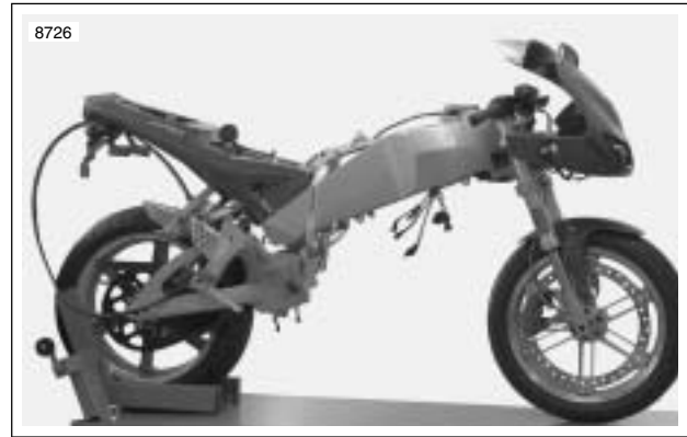
Figure 3-33. Rolling Chassis (Typical)
