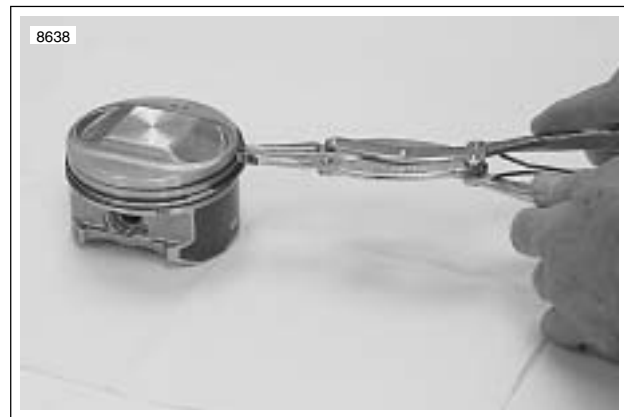
Figure 3-92. Removing Piston Rings
