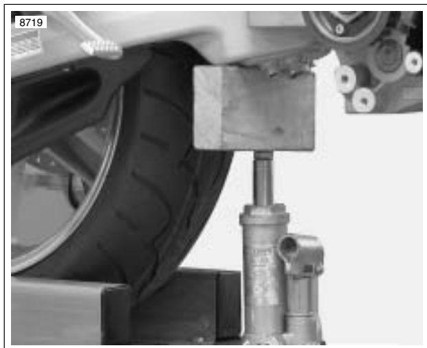
Figure 3-38. Supporting the Swingarm
