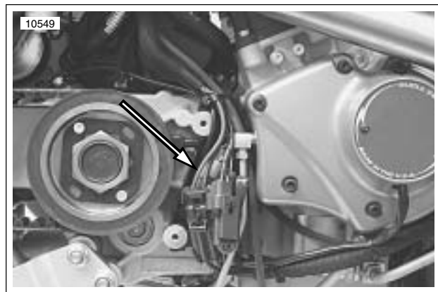
Figure 7-28. Positive Regulator Cable (red wire)
