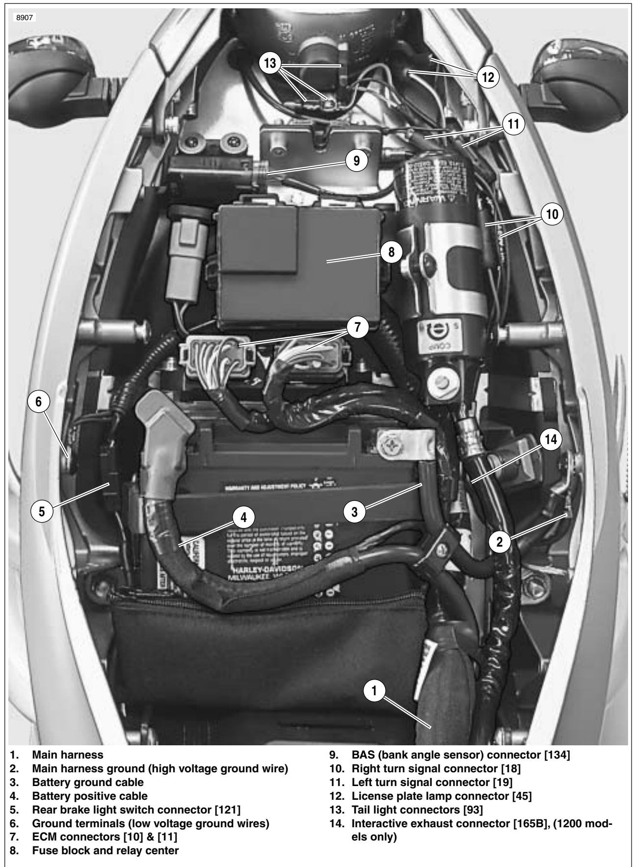
Figure 7-82. Main Harness and Electrical Connectors Under Seat
