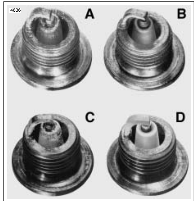
Figure 1-36. Typical Spark Plug Deposits
