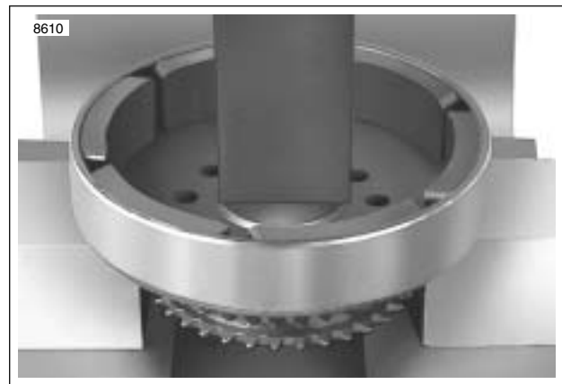
Figure 7-33. Removing Rotor From Sprocket
