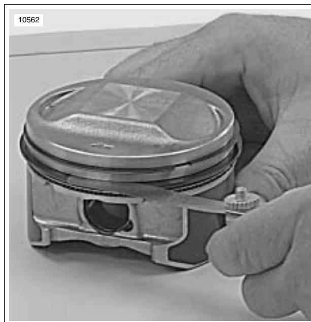
Figure 3-99. Measuring Ring Clearance in Groove
