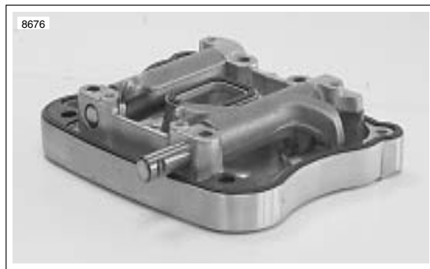
Figure 3-62. Removing Rocker Arm Shafts
