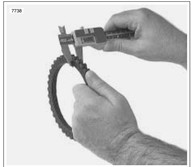
Figure 6-17. Measuring Friction Plates
