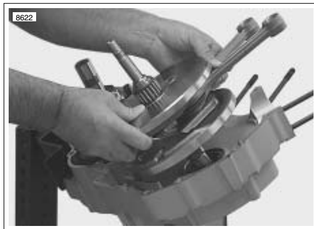
Figure 3-136. Removing Flywheels from Left Crankcase
