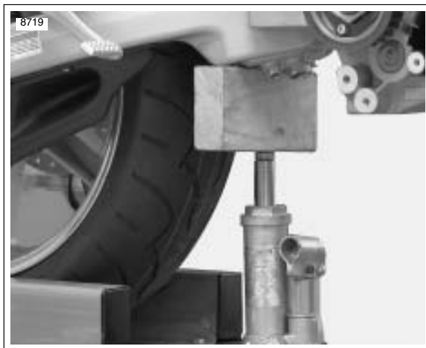
Figure 3-26. Supporting the Swingarm
