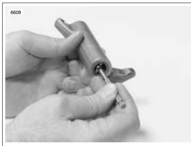
Figure 3-70. Measuring Rocker Arm Bushing Inner Diameter
