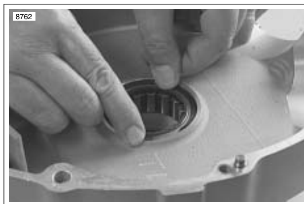
Figure 3-140. Removing Sprocket Shaft Bearing Retaining Ring
