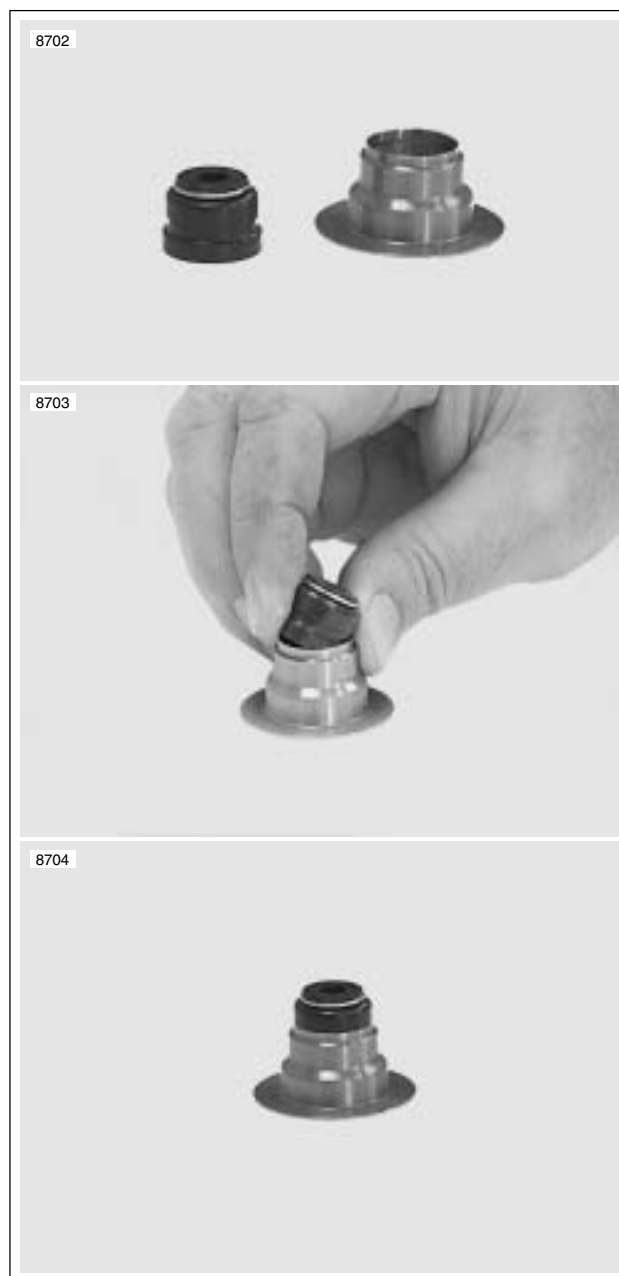
Figure 3-80. Valve Seal and Lower Collar Assembly (seal and lower collar replaced as assembly only)
