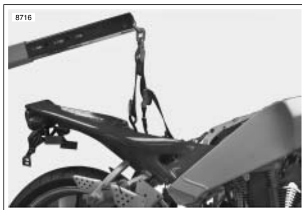
Figure 3-41. Supporting Vehicle for Assembly (Typical)
