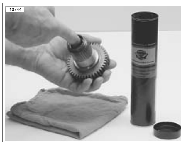
Figure 6-74. Lubricating Main Drive Gear Needle Bearings
