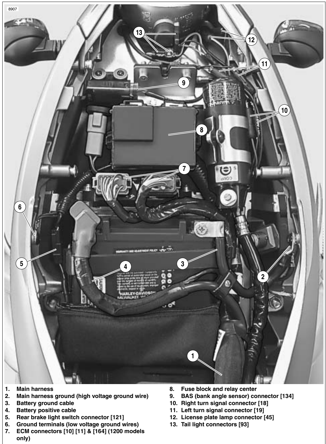
Figure 7-87. Main Harness and Electrical Connectors Under Seat
