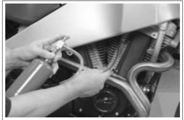
Figure 4-115. Checking for Intake Leak
