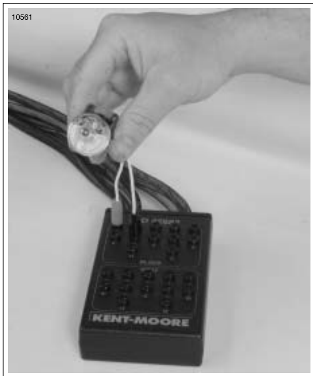
Figure 4-19. Ignition Coil Circuit Test
