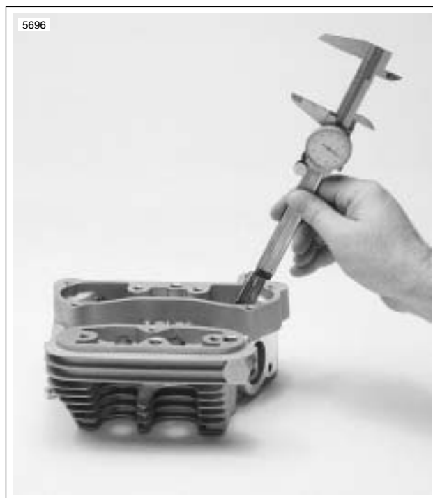
Figure 3-71. Measuring Valve Stem Protrusion
