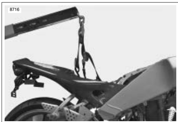
Figure 3-24. Supporting Vehicle for Disassembly (Typical)
