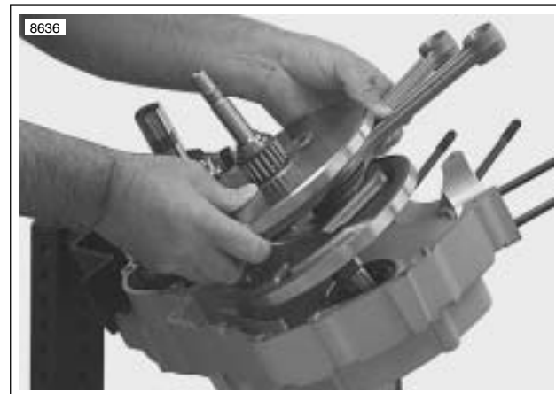
Figure 6-56. Removing Flywheels from Left Case Half
