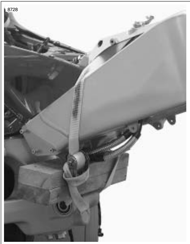
Figure 3-32. Securing Vehicle for Relocation (Typical)
