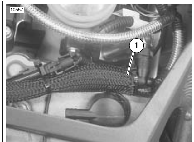
Figure 4-76. Engine Temperature Sensor Connector Approximate Location [90]
