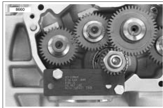
Figure 3-130. Crankshaft Locking Tool (Part No. HD-43984)
